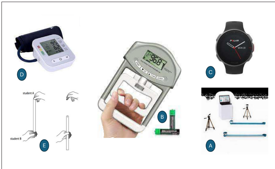
Figure 1: A) Optogait Measurement System; B) Hand Dynamometer; C) Polar; D) Sphygmomanometer; E) Test for Reaction Time
